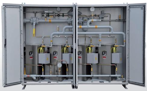
Version with multiple vaporizers (2 to 4 pcs. of size 100 kg/h or 170 kg/h) Max. total capacity 620 kg/h (4 x 170 kg/h)
