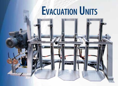
With an Evacuation Unit faulty filled or leaky gas cylinders can be emptied in a simple manner. The discharged medium is pumped into a storage tank.
